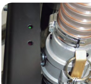
Attachment of a virtually indestructible RFID transponder on the coupling.
