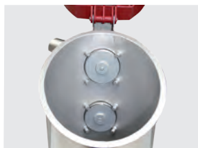
Pneumatic controlled material and vacuum valves
