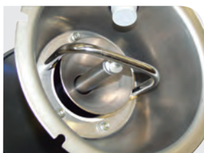
Pneumatic material discharge shut-off valve
