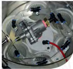
Filtration by (6) Urethane coated Polyester filtration elements
