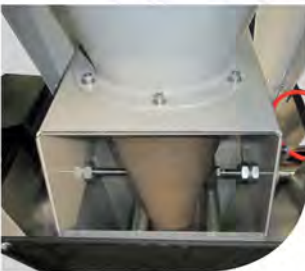
Pneumatically actuated discharge for accurate control of weigh discharge.
